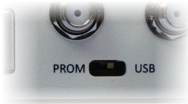
Programming switch on real panel
